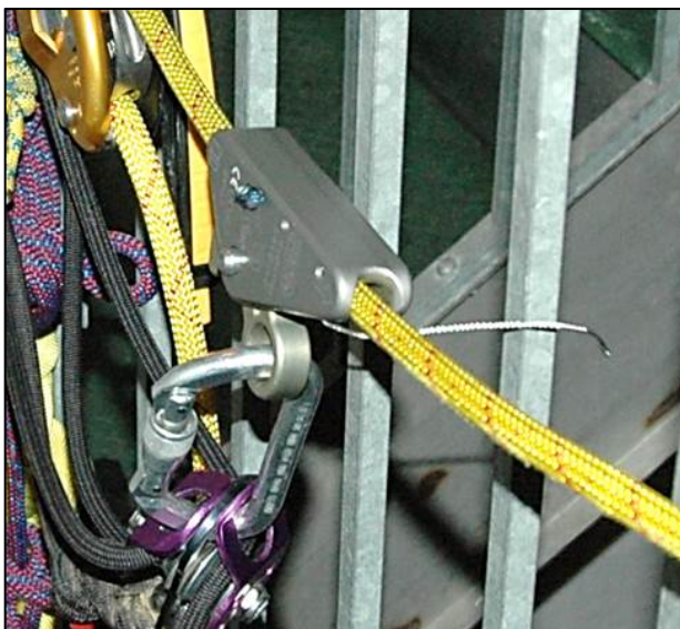
Figure 8- Damaged Rescucender showing broken retention wire.
