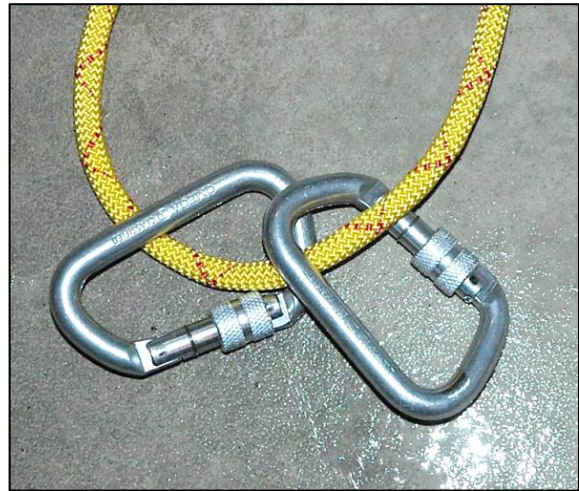
Figure 7- Carabiners, used for high directional, on the main line following the accident.
