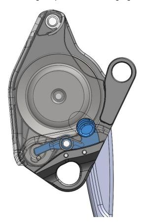
1. **Open the Moving Sideplate**. If the Side Plate Release Latch is difficult to actuate, the latch can also be operated by pressing down on the latch-stop feature accessible through the sheave window of the sideplate (see orange arrow below).
