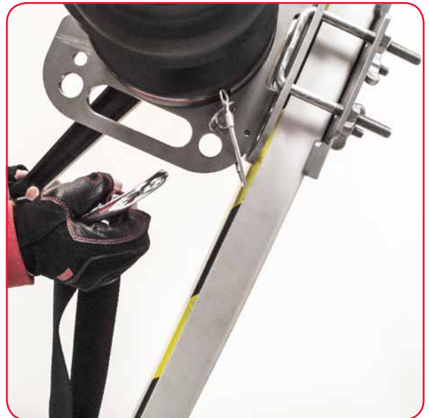
7. Engage the connector and the anchor device to the plate on the winch side, and to a safe anchorage point on the opposite side.
