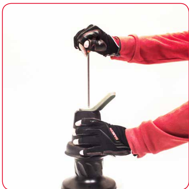
3. Tighten the control lever screw.
